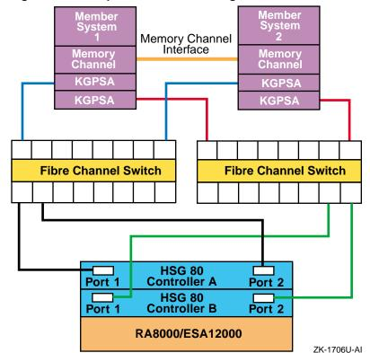
Figure 6-5: Multiple-Bus NSPOF Configuration Number 1
